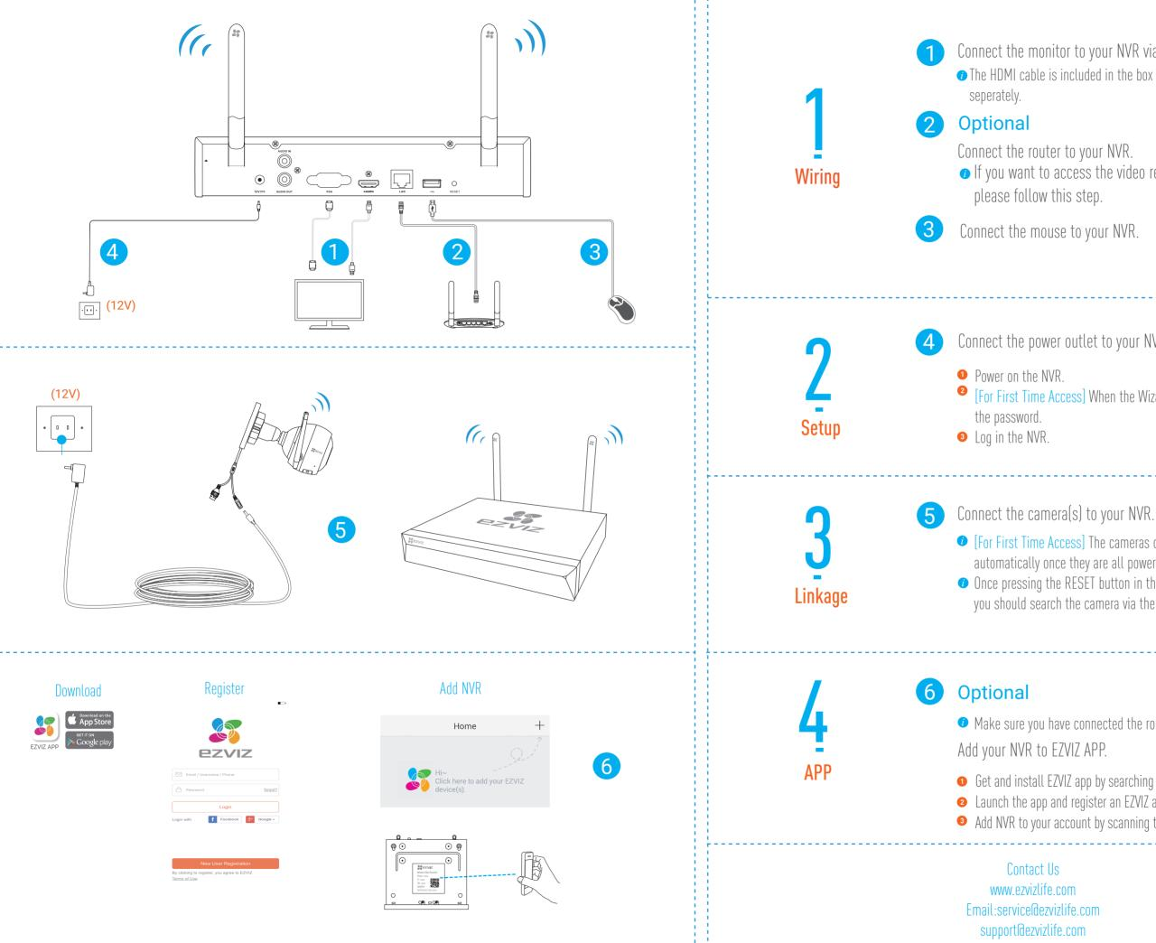
Connect the monitor to your NVR via the HDMI or VGA cable. • The HDMI cable is included in the box while the VGA cable should be purchased
